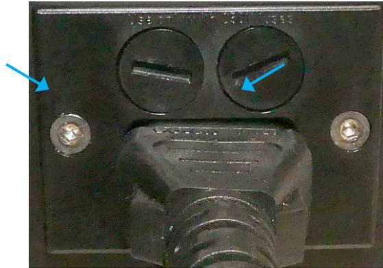
Figure 2: Position of fuses
