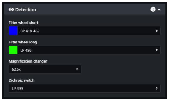
Select the desired magnification in the Detection box.
