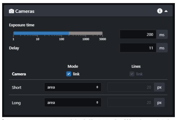
Set camera exposure to get a good signal without saturation. 200 ms is a good starting point.
