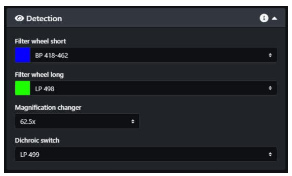
Select the filters that give the clearest signal on the camera feeds.
