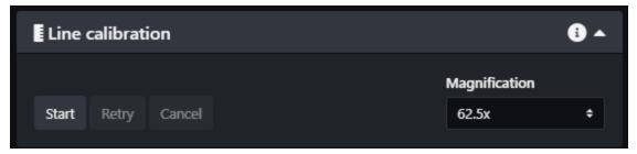
Use the Line calibration box to sync the rolling shutters to the scanning beam. Click Start and check the auto alignment results.
