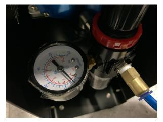
Check that the gas pressure gauge under the table reads 1 bar.
