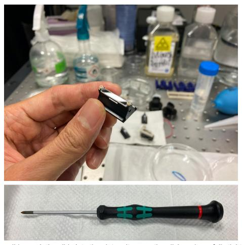
If using glass slide, push the slide into the slot on its mounting dish and carefully tighten the screws.
