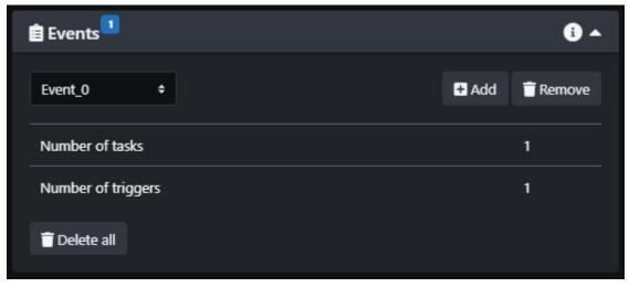
Add an Event, which is an experiment with a set of tasks and triggers.
