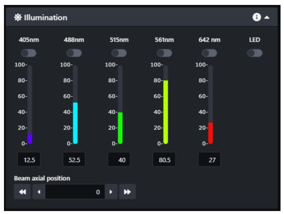
Turn on the laser you will be using for the experiment. Use high laser power to get a better signal for calibration. If you are using lasers from 488 nm to 642 nm, you only have to calibrate one of them. If using 405 nm, calibrate it separately and save the adjustments in a separate channel.
