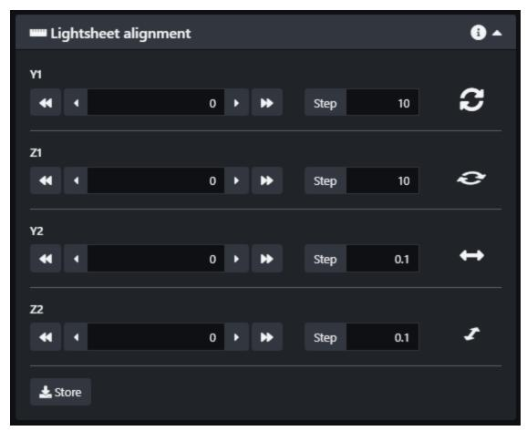
Focus the beam using Z2, then center it left-right using Y2. Y1 and Z1 should not need adjustment. Once done, click Store.
