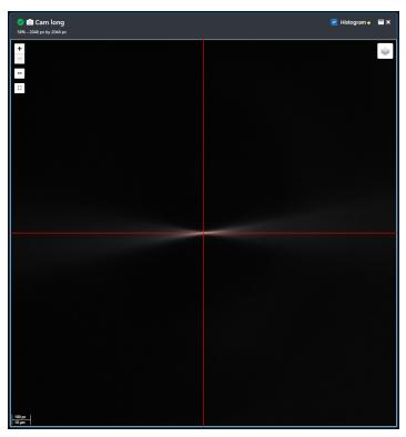
For centering adjustments, turn on the crosshairs by clicking the white button at the upper right corner of the camera view.
