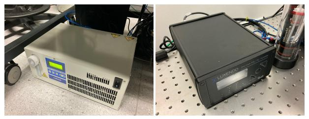
Turn on the temperature (left) and gas (right) controllers. The switch for the gas controller is on the back.
