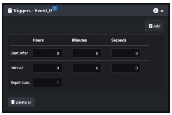
Define the triggers. This is where you can set time lapse. Set all timings to 0 and Repetitions to 1 if there is only one time point. If timings are set to 0 with multiple Repetitions, the system will repeat acquisitions as fast as possible.
