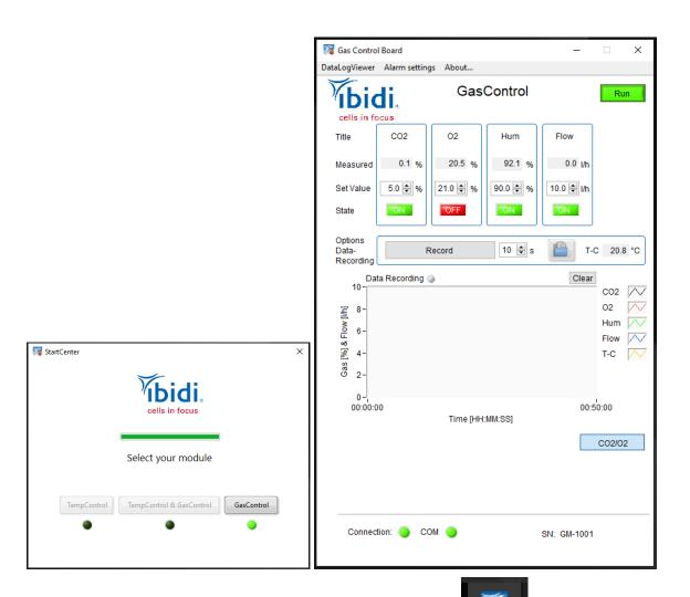
To set carbon dioxide and humidity, launch IncuControl software and click "GasControl" (left). Set the desired conditions (right) and click the top right button to run or stop the gas control. When the button shows "Run" in green, it is running. When it shows "Stop" in red, it is stopped.
