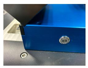
Remember to press the laser interlock button to reactivate laser.
