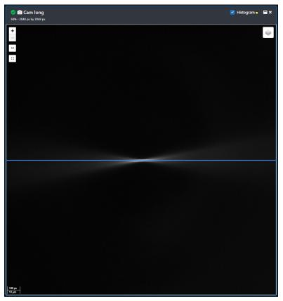
Click Retry if the blue line doesn't coincide with the beam. Once aligned, click to the next step.
