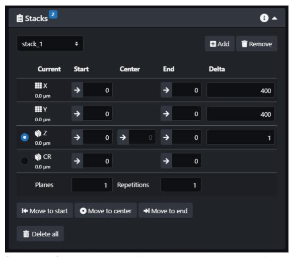
If applicable, define z-stack and xy tiles. Move the sample and assign the travel limits by clicking the appropriate arrows.
