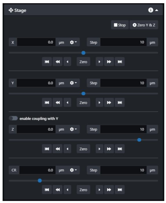
Find the sample using the stage controls. CR (refractive index compensation) should be left at 0 for most aqueous imaging media.
