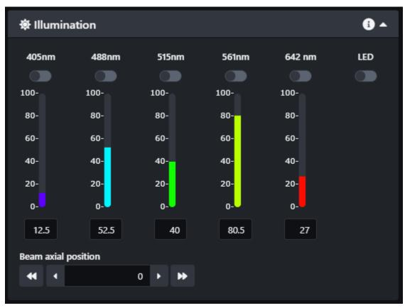
Turn on the sample chamber LED using the switch at upper right of Illumination box.
