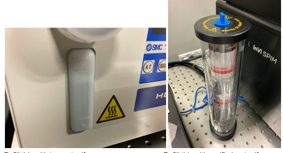
Refill this with tap water if necessary. Do not use purified water.
