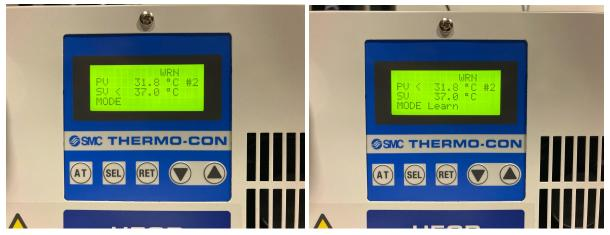
To set temperature, press "SEL" button to choose "SV" (left). Press up/down triangle buttons to set temperature. Press "RET" button and check that the bottom of the display shows "MODE Learn" (right).
