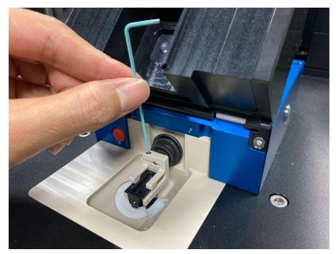
Gently slot the sample holder into the stage pin. Do not force it as the stage pin may be pushed out of position. Tighten with the light blue hex key.
