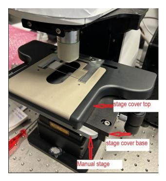
You may put the stage cover upside down on the optical table after removing it from the manual stage.
