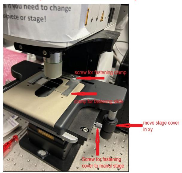
When mount the stage cover, please align its base and top rear side to the rear side of the manual stage.
