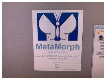
Launch MetaMorph software. Watch for the MetaMorph logo to appear in the software window (above). If it doesn't appear, it hasn't detected the camera and you have to restart the computer.
