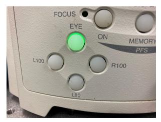
Press the EYE button on the microscope if you want to use the eyepieces, or L100 if you want to view image on camera.
