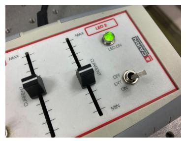
On the LED control panel, flip the right-hand switch to EXT for control using the software (below), or ON if you want to control it directly from the panel. The right-hand black slider controls brightness.
