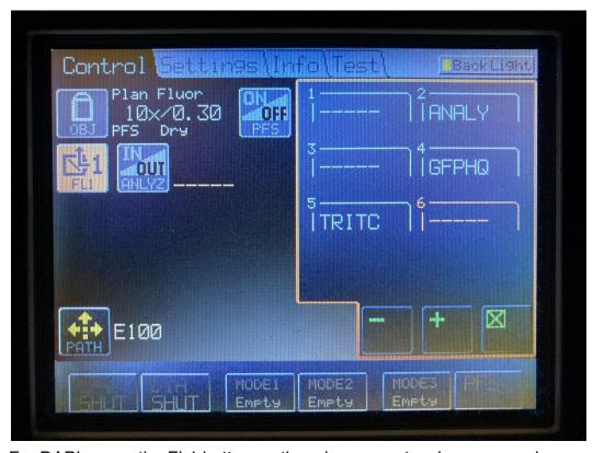
For DAPI, press the FL1 button on the microscope touch screen and press position 6.
