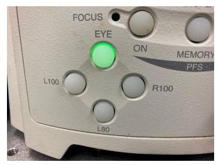
Press the EYE button on the microscope if you want to use the eyepieces, or L100 if you want to view image on camera.
