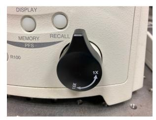
This knob on the front of the microscope should be in this position (1x).
