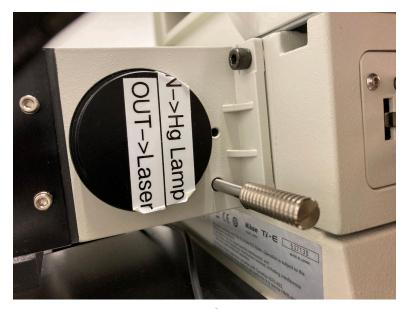
Push in the pin at the back of the microscope.
