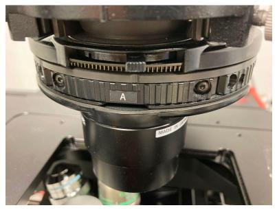
Swap in the bright-field condenser if necessary. Remember to align the notch at the back so it doesn't rotate, and tighten the set screw securely. Rotate condenser turret to position A.
