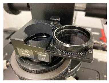
Polarizer should be out of the light path.
