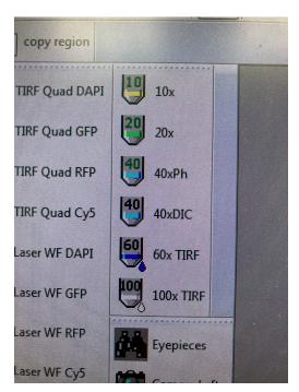
Select objective in the software (instead of the microscope touch screen) so the software will embed the correct scale information in the image.
